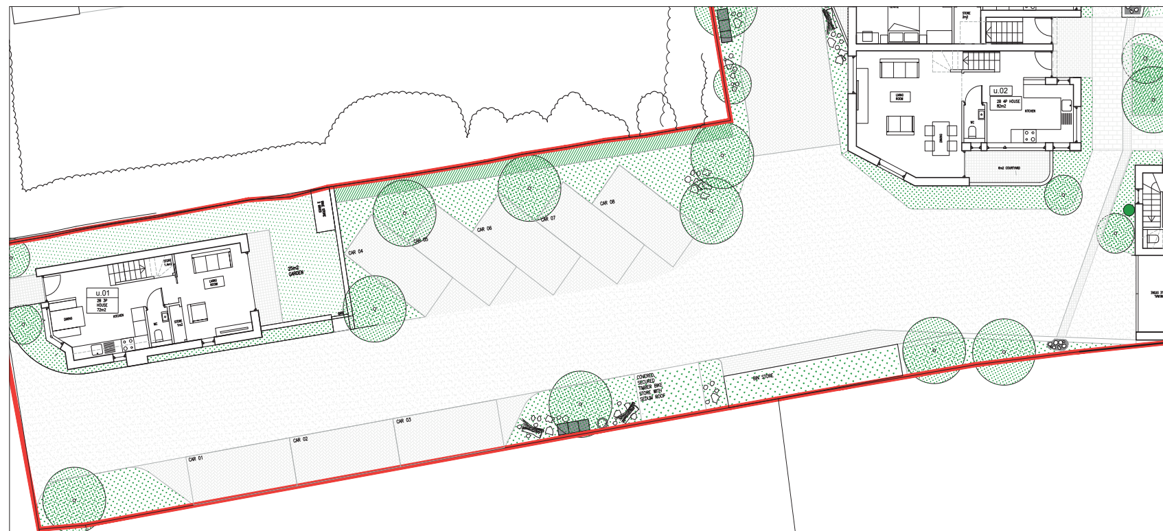
Revised scheme with the refuse truck access revised to reduce the width of the hardstanding. Parking numbers reduced and significant additional planting and landscaping added
