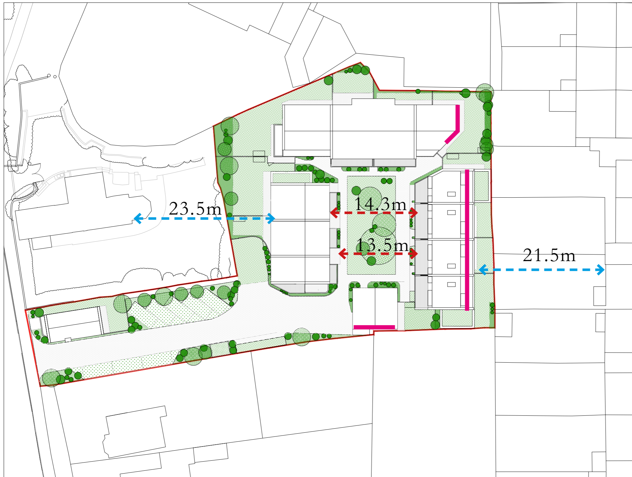
Figure 18: A minimum distance of 21 metres will need to be maintained between a rear extension of up to two storeys and the rear windows of an opposing dwelling. This will avoid potential privacy and overlooking issues.
