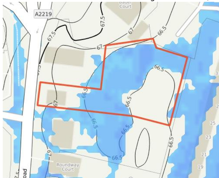
Figure 1: Risk of Flooding from Surface Water Flooding (1 in 1000 year event) from EA data, in relation to existing contours.
