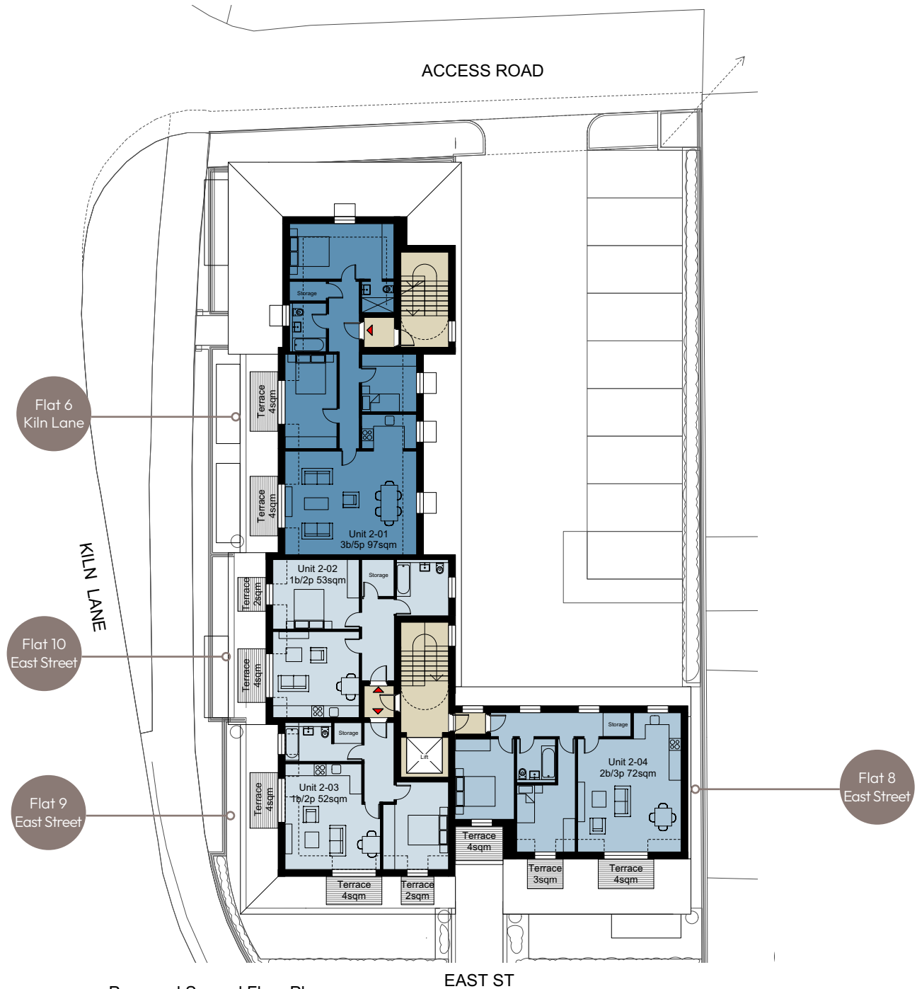
2 Proposed Second Floor Plan Scale: 1:100
