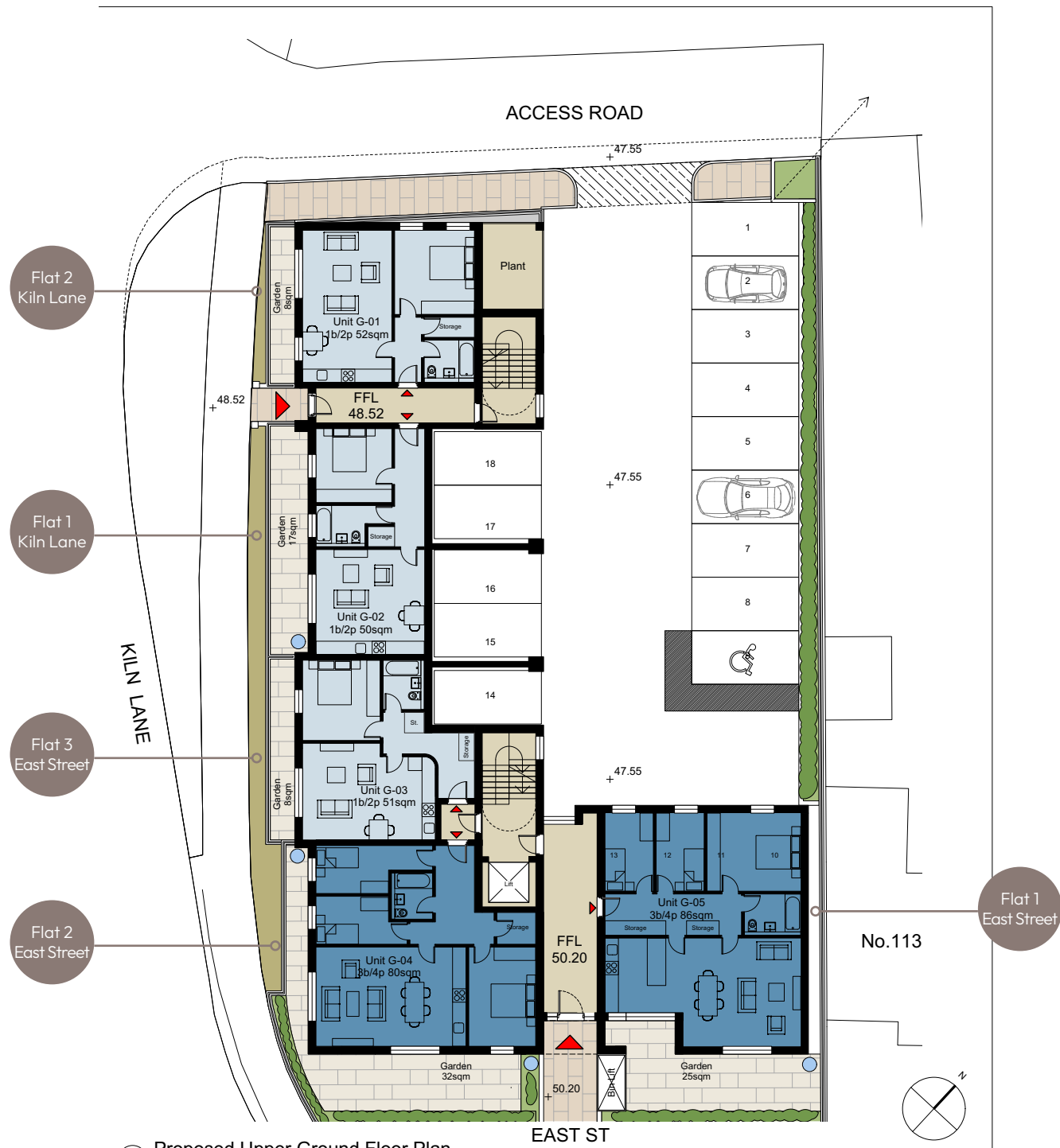
2 Proposed Upper Ground Floor Plan Scale: 1:100
