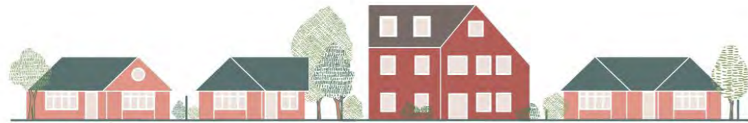
Figure 2.10d: Where surrounding buildings are predominantly single storey, new development should seek to accommodate a third storey within the roof space.
