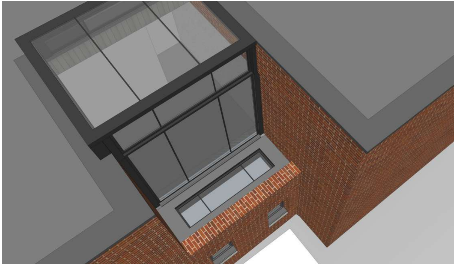
3.15 Proposed lightwell and stepped back facade to allow additional daylighting. Introduced in pre-application 02.
