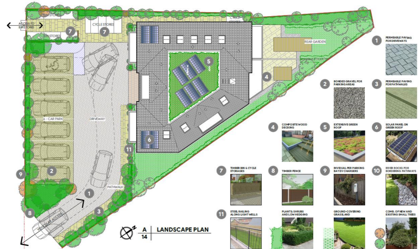
Figure 16 – Landscape Plan of the proposed development at 260 Coombe Lane showing the existing shrub and plants at the front garden to be retained; the supplementary shrubs/low hedging, and small, narrow trees for both the front and rear gardens; the extensive grass lawns on which these planting shall be placed; permeable pavers for the driveways and pedestrian pathwalks; and the extensive Green Roof
