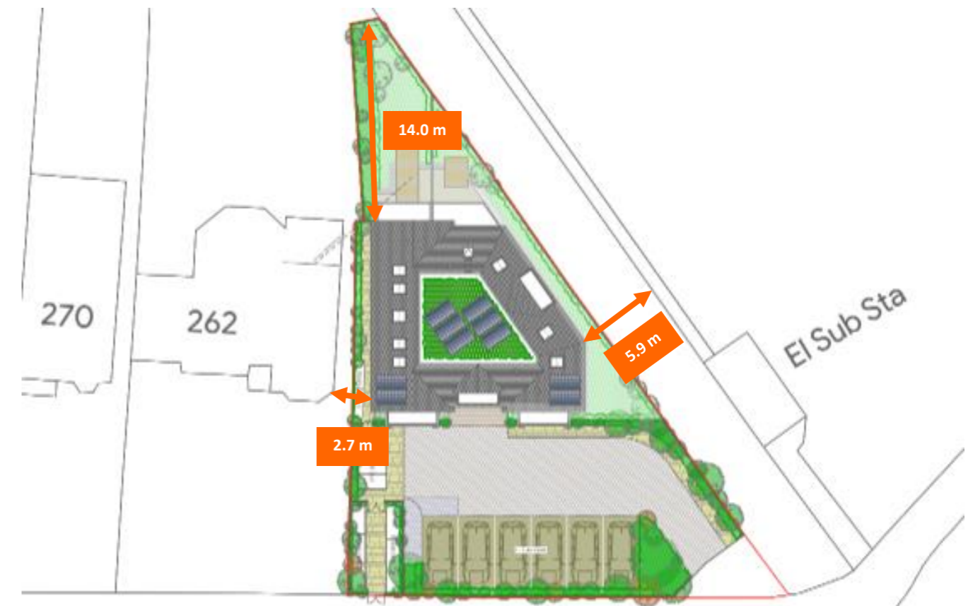
Figure 11 – Proposed Block Plan of 260 Coombe Lane showing how much the proposed development is setback from the boundaries shared with neighbouring properties
