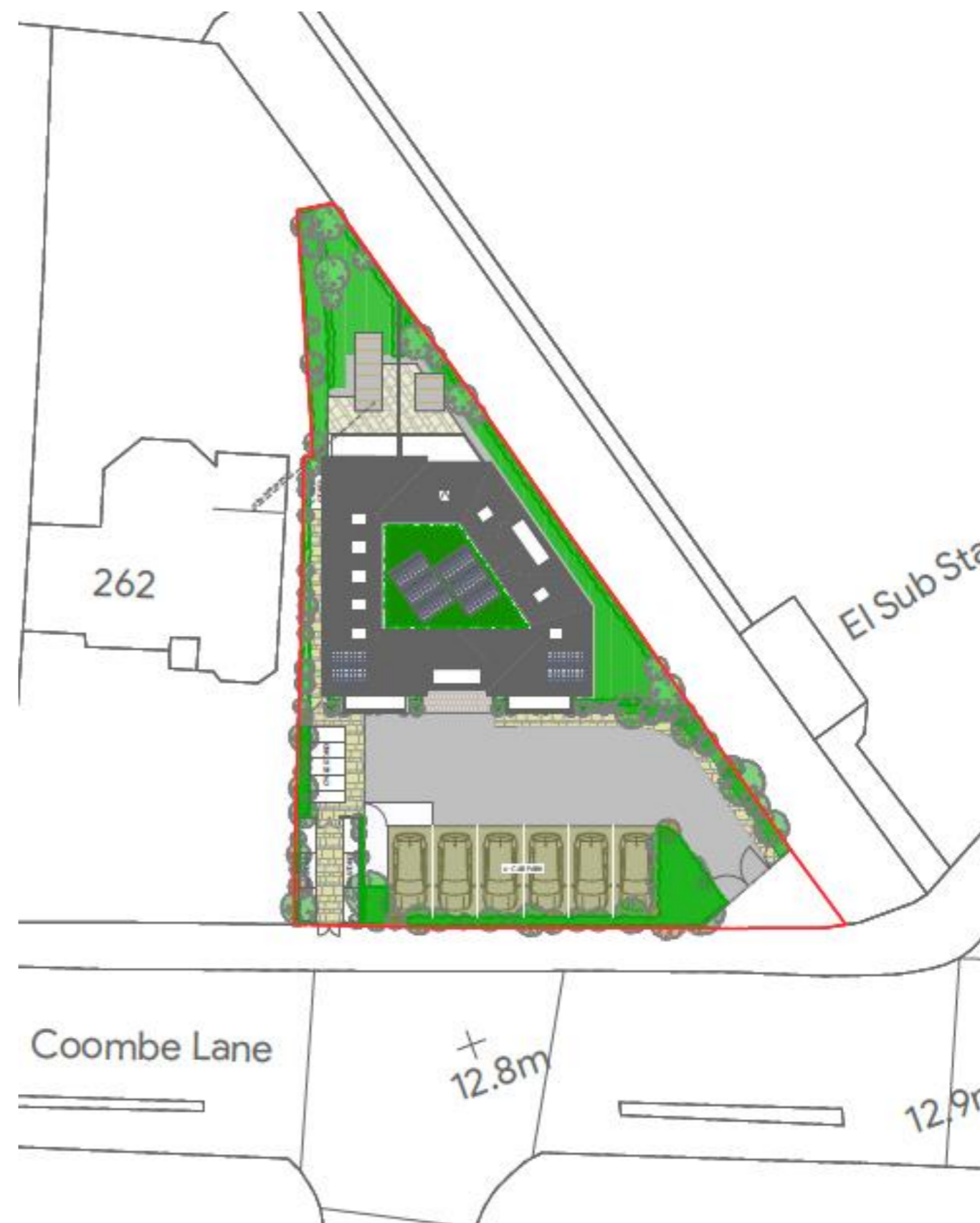
Figure 4 – Proposed Block Plan of 260 Coombe Lane for demolition of existing bungalow, and erection of a two-storey dwelling with accommodations at the basement and roof space levels comprising six (6) self-contained flats
