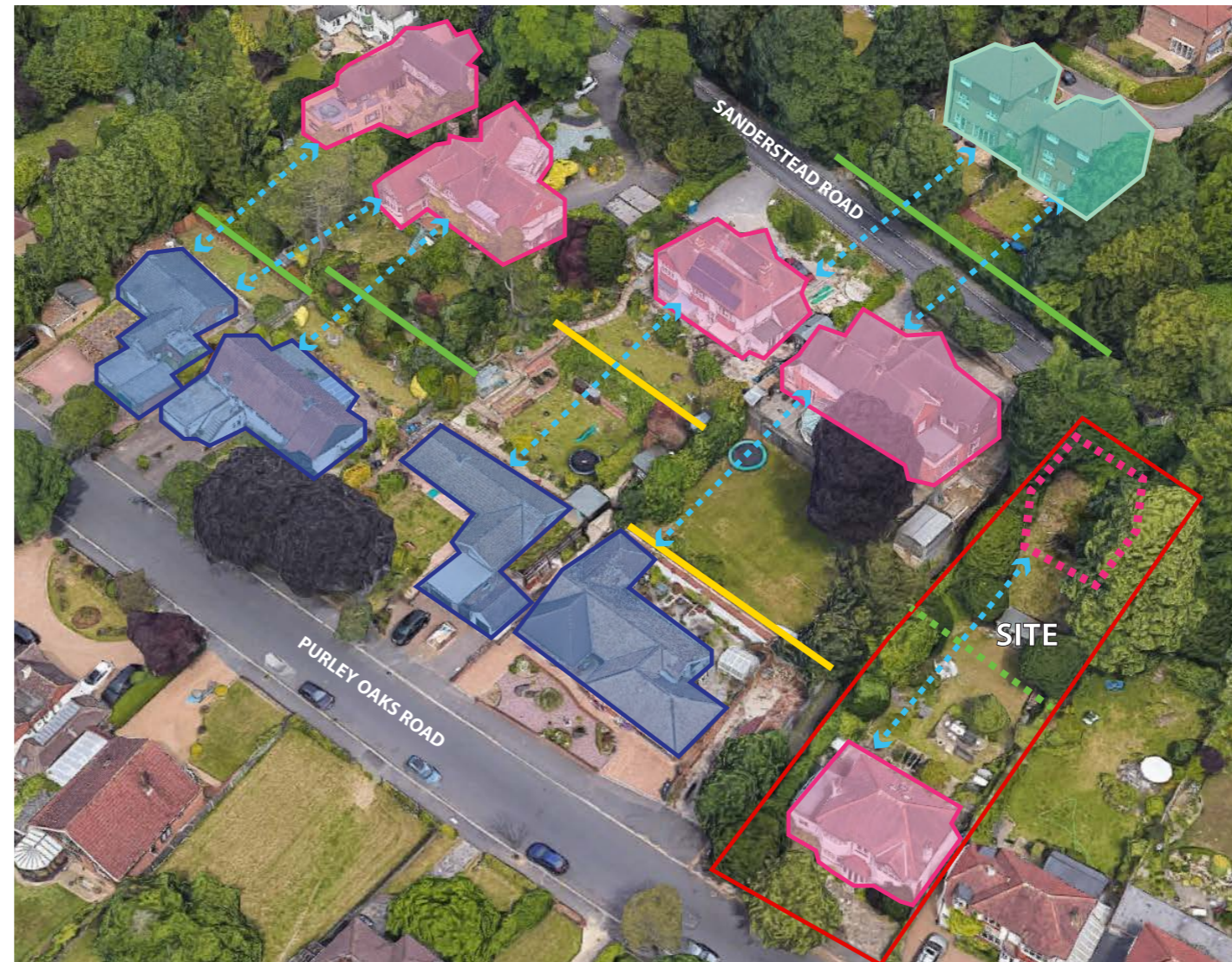
Birds eye view diagram showing building heights, distances between opposing windows and boundary vegetation
