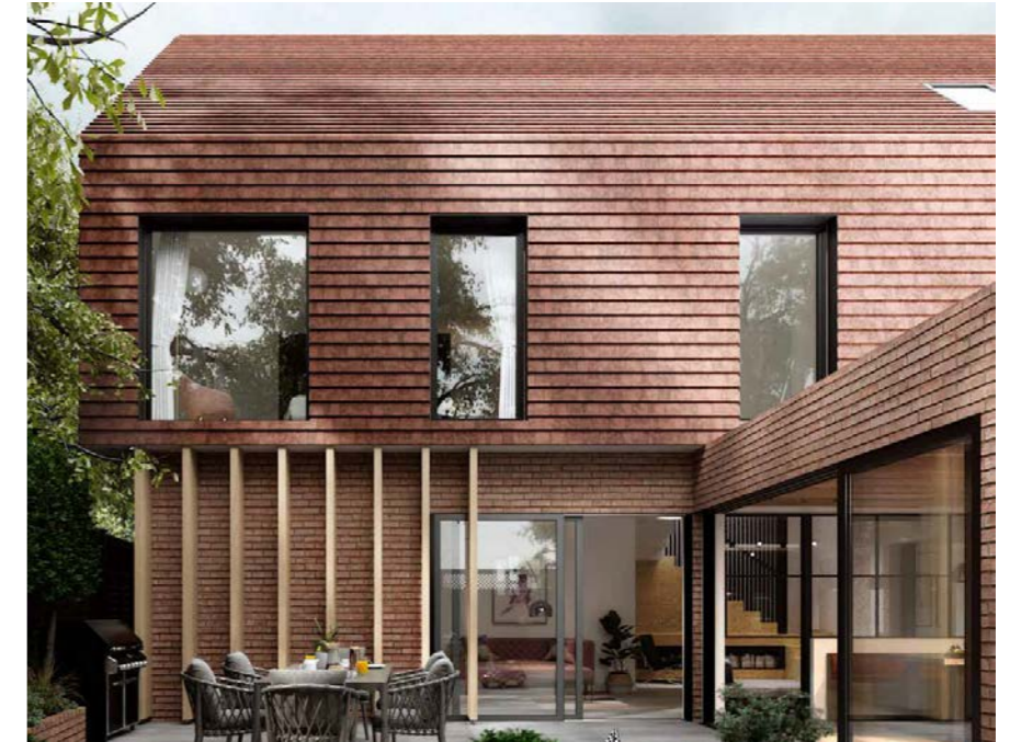
Terracotta House by Our Studio Contemporary use of terracotta tile hanging and tiled roof
