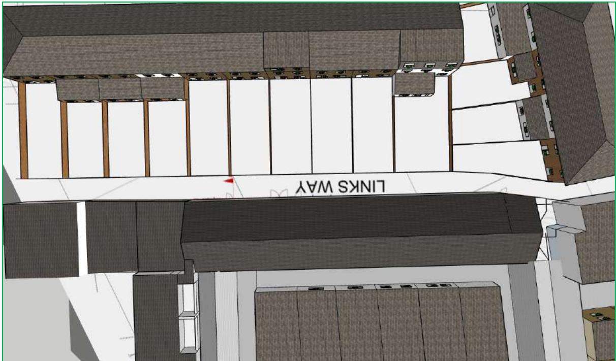
Figure 8: Shadow Analysis for September 21st at 4pm
