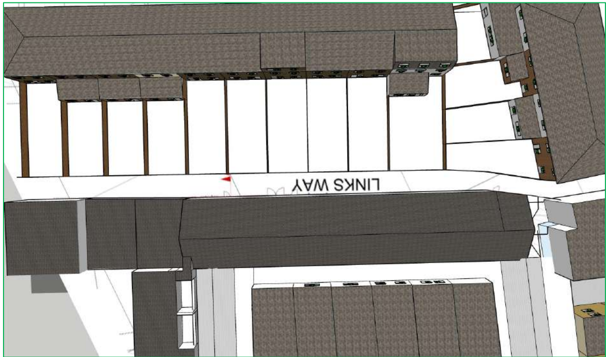
Figure 5: Shadow Analysis for June 21st at 10am
